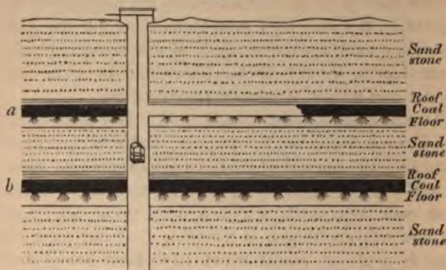
Imaginary section of a coal-mine.
